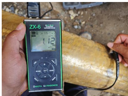
检测腐蚀程度为72%，现场验证实测腐蚀程度为77%
