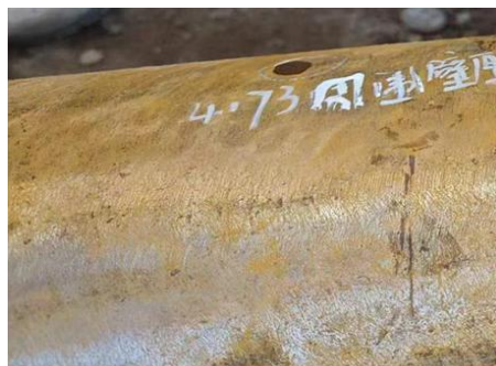
检测腐蚀程度为72%，现场验证实测腐蚀程度为77%
